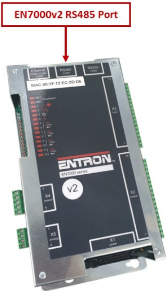
Figure 14: EN7000v2 Control RS485 Port
